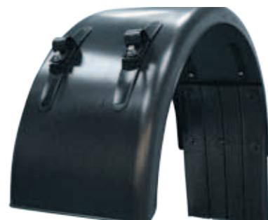
Antispray **SPRAYFLEX®** and composite bolts and nuts system **CUPFLEX®**
