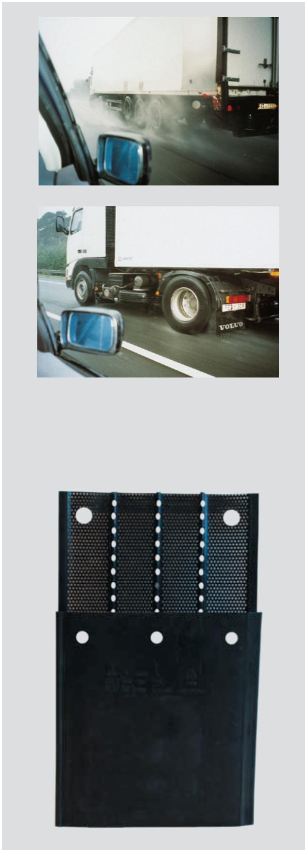
**SPRAYFLEX®** is available with or without logo, fitted on the mudwing or prepared for fast assembly to suit your production.
